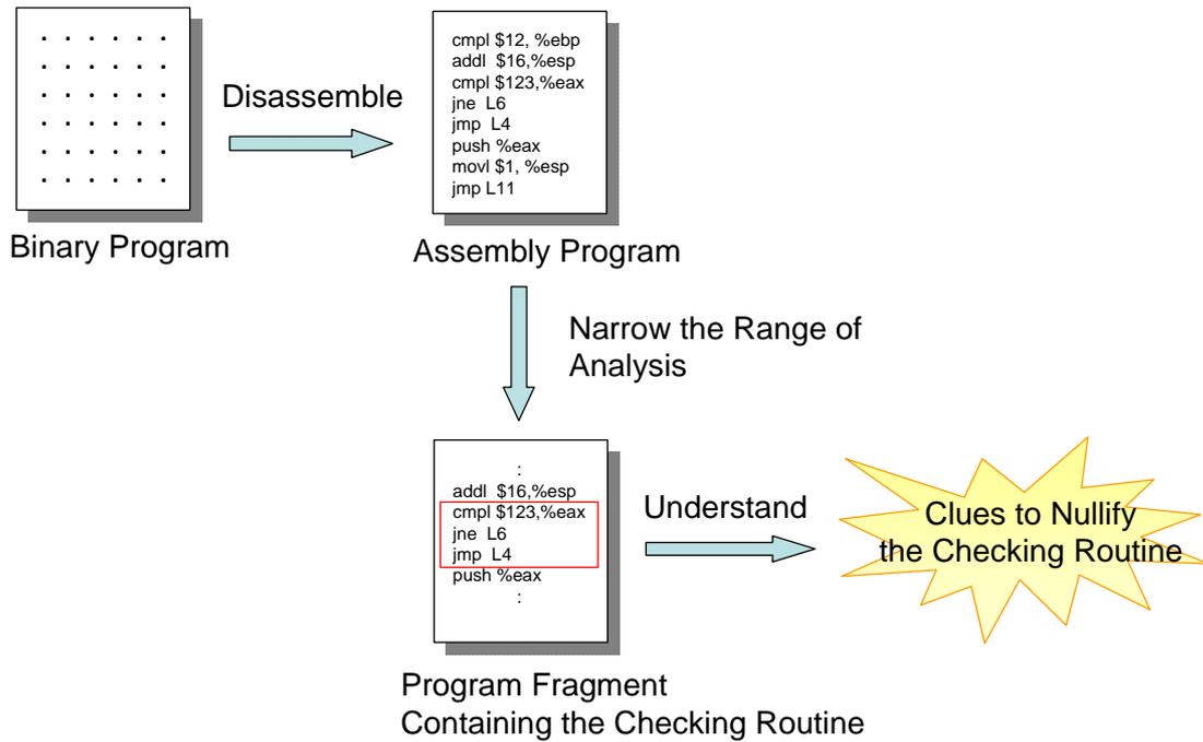
Figure 1.2. A scenario of obtaining clues to nullify the password-checking routine and the program may be used without password authentication. As seen in this example, whenever software is reverse engineered, there must be a process where an attacker reads the program and tries to understand the program.
